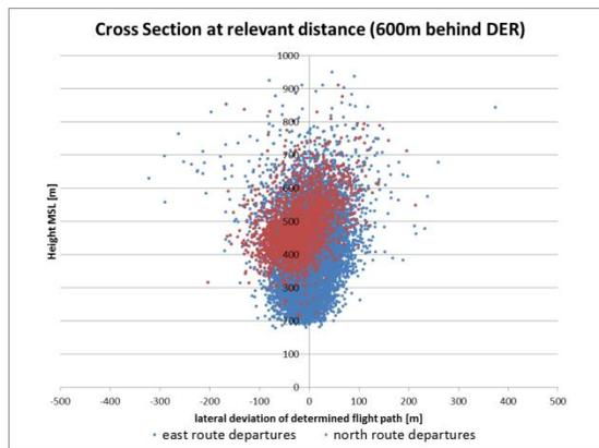
Figure 14. Relevant Cross Section passing through the critical obstacle, at 600m DER distance, departures from runway 07C
