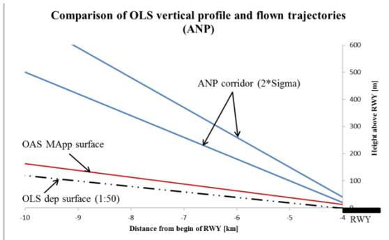
Figure 3. Heterogenous safety margins resulting from OLS and OAS (departure)
