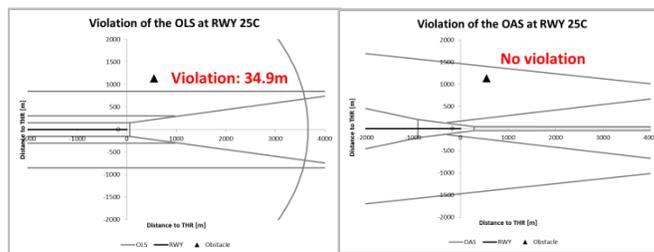
Figure 12. Excerpt of the Obstacle Clearance Analysis for the runway 07/25C, OLS – left figure, OAS CAT I – right figure
