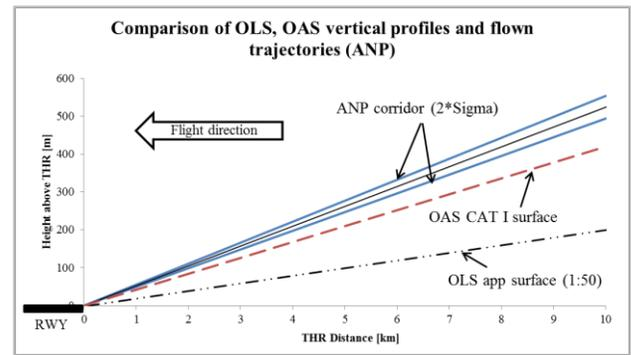
Figure 2. Heterogenous safety margins resulting from OLS and OAS (during approach)
