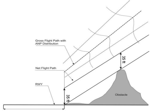
Figure 4. Additional Obstacle clearance and required net flight path corrections resulting in lower CR as for OLS and OAS
