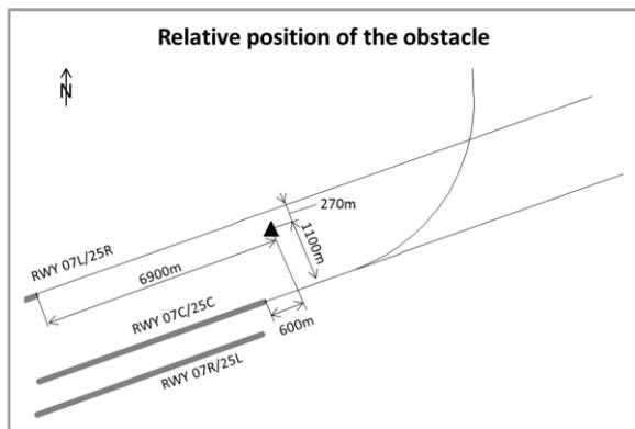
Figure 11. Location of the critical obstacle - the safety case EDDF
