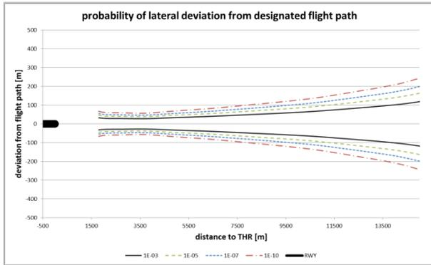
Figure 7. Probability of lateral deviation from designated flight path or risk to hit an obstacle with  $CR(z)=1$  in lateral plane
