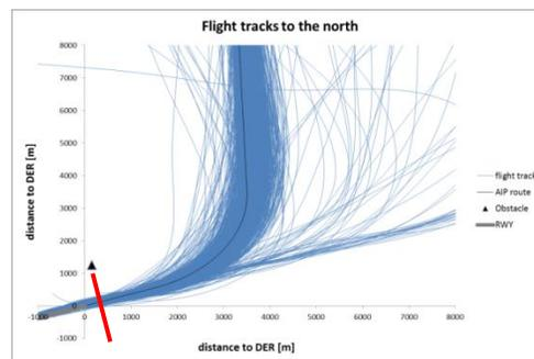
Figure 13. FRA Flight tracks for runways in use 07, outbounds, FANOMOS Data, with obstacle critical cross section (red line)
