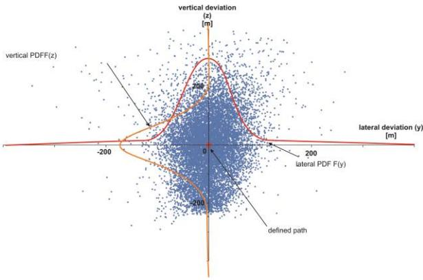
Figure 6. Normally distributed track offsets around the flight path
