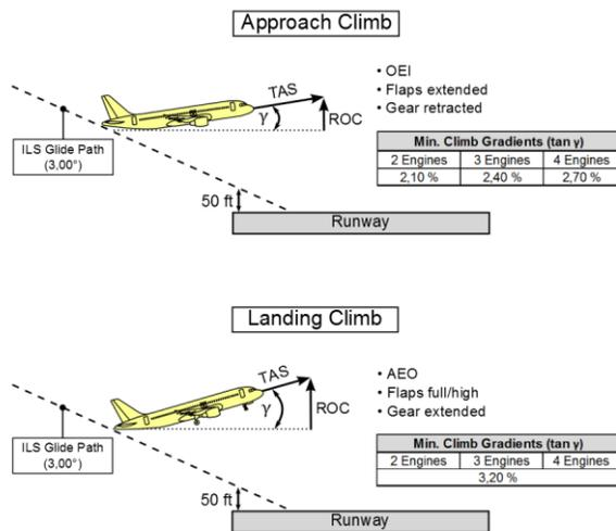
Figure 9. Worst Case Analysis for Approach and Landing Climb obstacle clearance: Approach/Landing configuration impact on ANP and Rate of Climb
