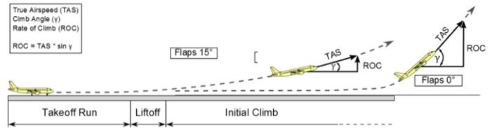
Figure 10. Lowest pass altitude analysis for takeoff obstacle clearance
